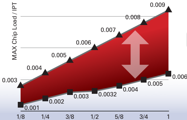
K Cast Iron Python – Chip Load Operating Range "K" Cast Iron ■ Min IPT "N" ▲ Max IPT "N"
